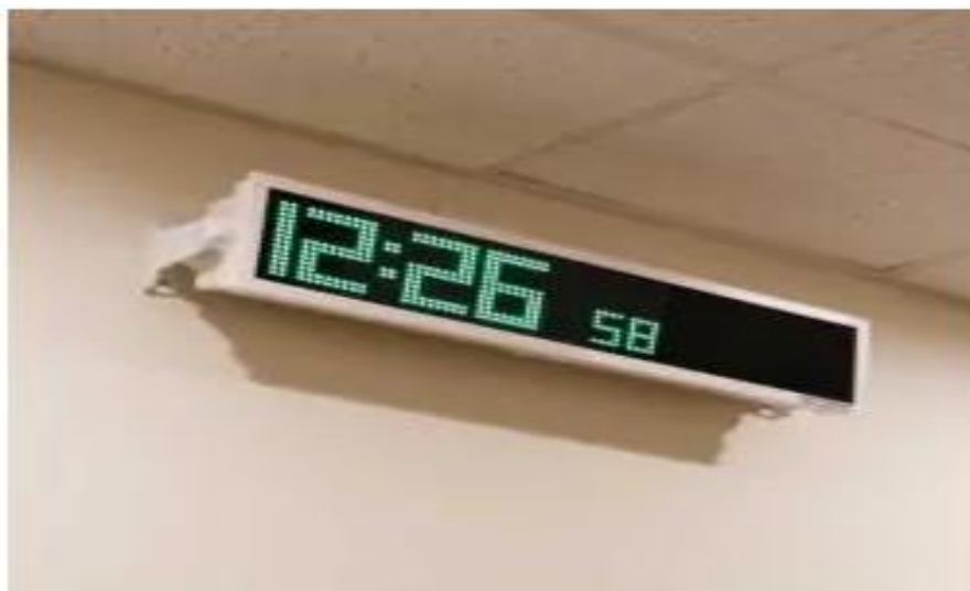
Figure 2: Modern Wireless LED Message Board: For Text Messaging and Digital Time Display
