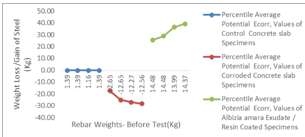
Figure 3.7B: Average Percentile Rebar Weights- After Corrosion (Kg) versus Weight Loss /Gain of Steel (Kg)
