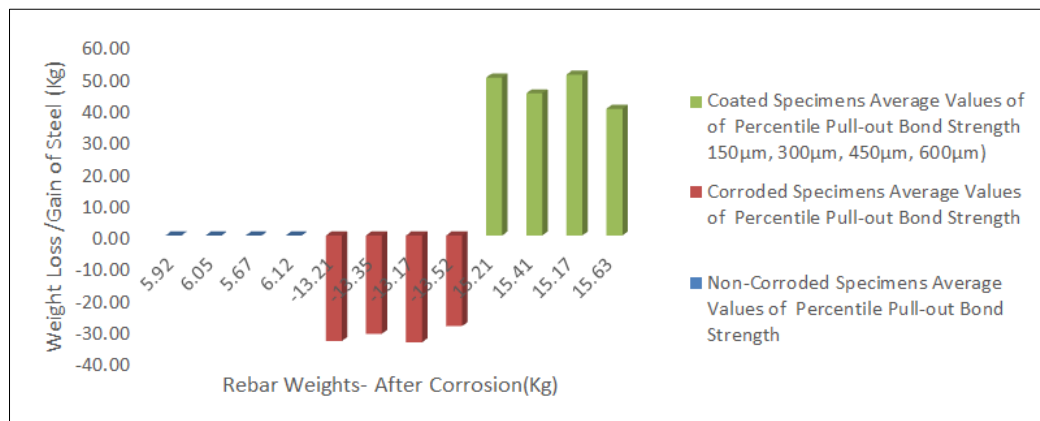
Fig. 6b: Average percentile Rebar Weights- after Corrosion versus Weight Loss /Gain of Steel
