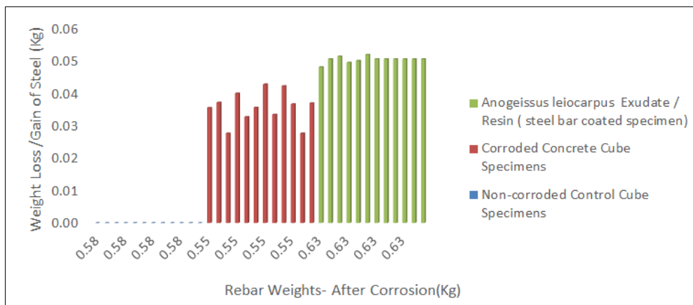
Fig. 6: Rebar Weights- After Corrosion versus Weight Loss /Gain of Steel
