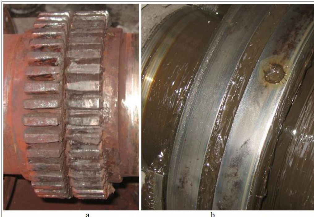
Fig. 8: Wear of the half-coupling (a) and signs of rotation (b) of the outer ring of the induced draft fan bearing
