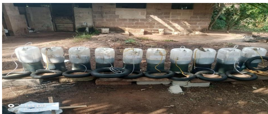
Fig. 2: Batch A showing the ten fabricated digesters with gas in the tubes
