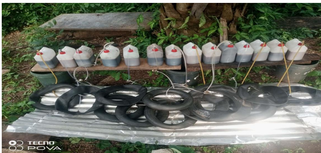
Fig. 4: Batch C for kinetic modelling of biogas production
